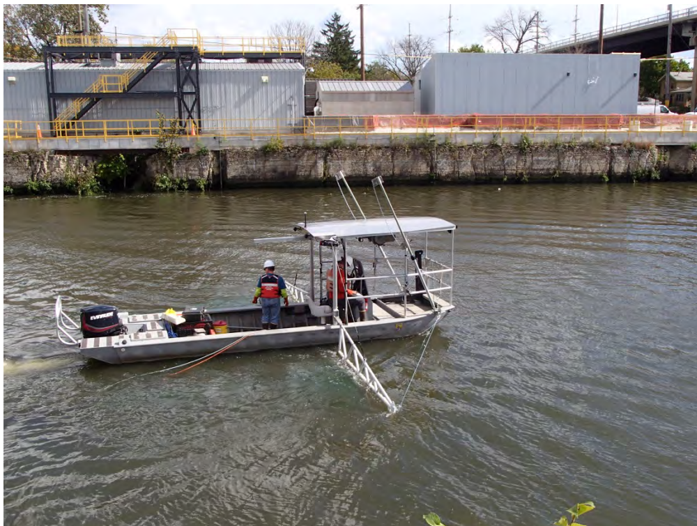
Figure 5. Paupier butterfly trawl net deployment used to capture fish within the vicinity of the CSSC electric dispersal barriers. The nets extend over the sides of the vessel and are lowered and raised into and out of the water at precise locations.
