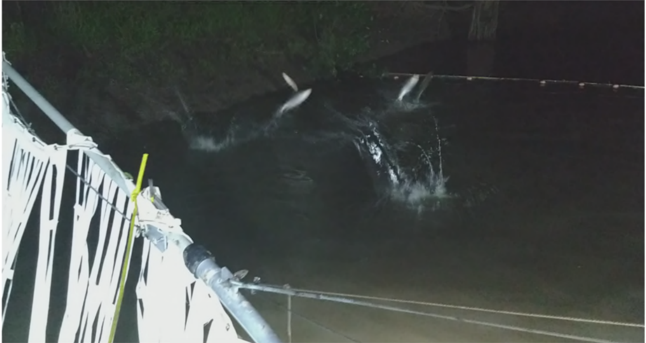
Figure 7. Scare curtain driving fish up a ramp net into an opening on the surface. Net has a floor and back to prevent escape once fish enter. Lighted scare curtain deters fish from swimming back upstream.
