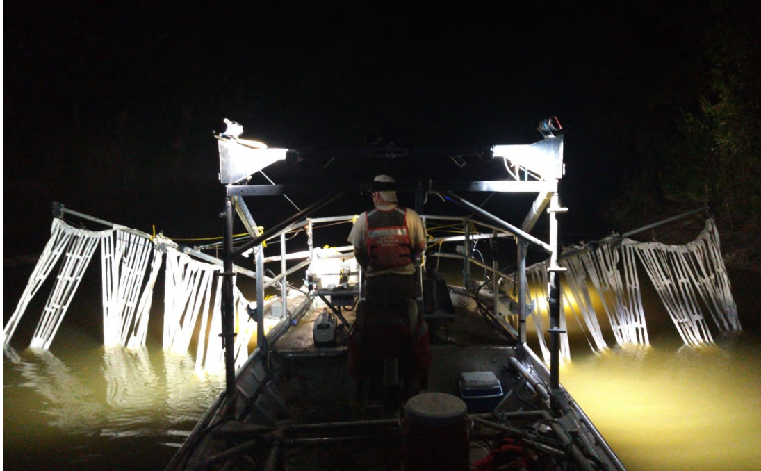
Figure 1. Boom and front mounted flexible “Scare Curtain” used with high intensity LED lights in a small tributary
