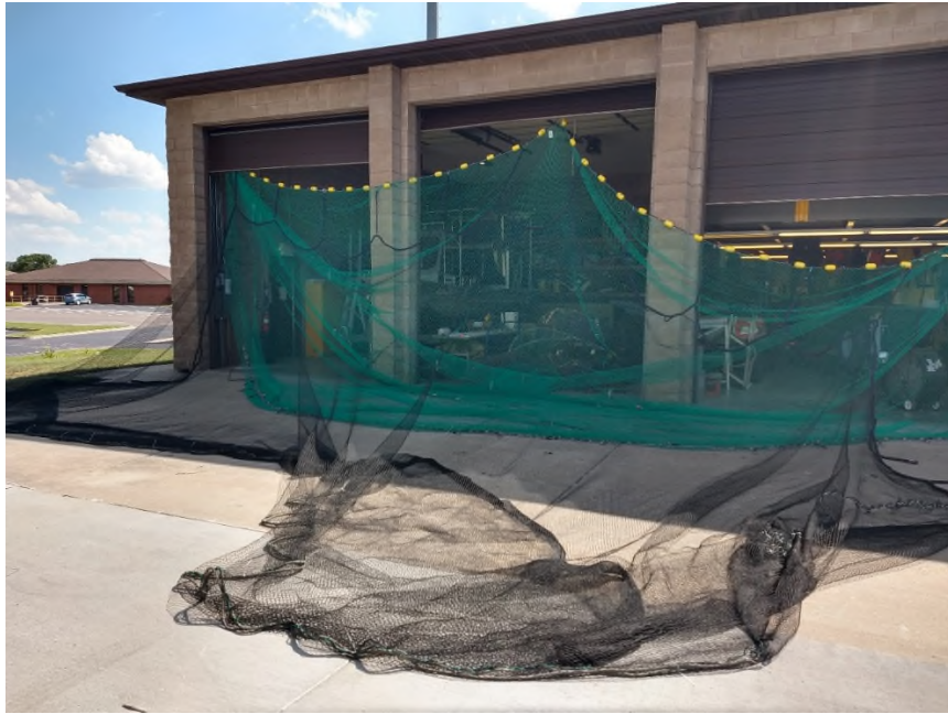
Figure 3. Ramp net prototype. Black netting is angled forward and anchored the bottom substrate. The black polyethylene netting floats creating a ramp to the surface where a 1m gap connects the green funnel net. The entire net is enclosed except for a gap at the top, which the fish jump in, and funnel bag to remove the fish.
